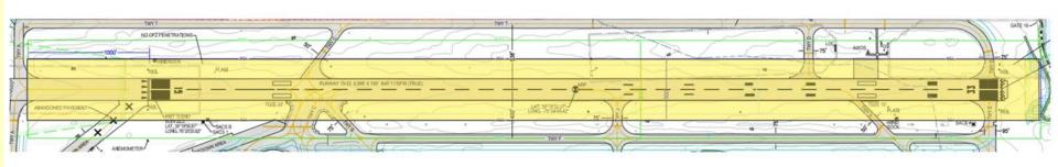
• Safety Areas, Runways, and Taxiways, are surrounded by safety areas that are designed to provide an increased level of safety for aircraft landing and taking off. The dimensions of the safety areas vary according to the runways (RWY 15-33 - 250' each side of centerline – image above). These safety areas are intended to minimize damage to an aircraft during emergency situations, such as an aircraft overshooting or veering off the runway.
